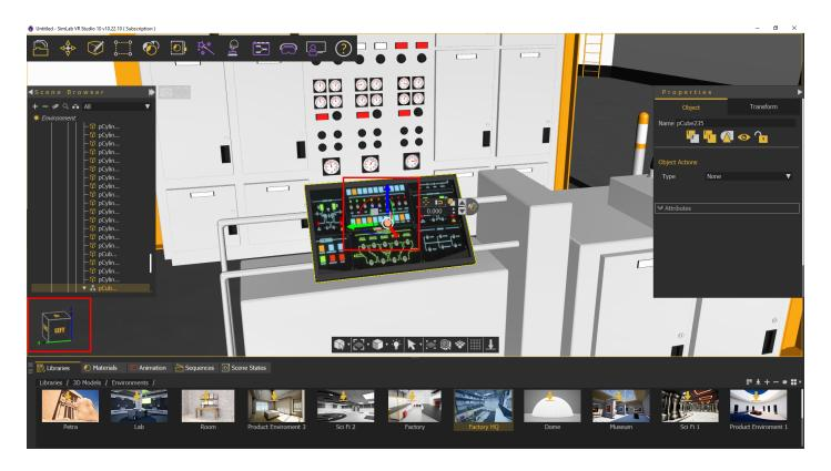
When the user clicks any dragger, a small scroll combo box will appear in the **Quick Access Toolbar.** The user can use this box to input exact numbers for translation/rotation/scale or can just scroll up and down. If the user prefers to freely drag
