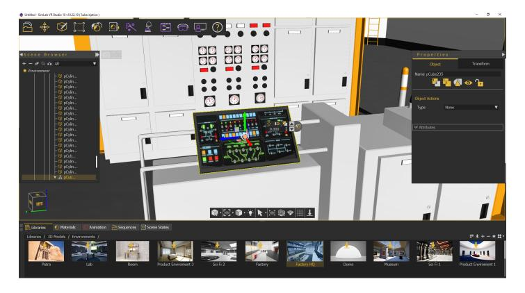
**Global Transform:** Displays transform axes on the selected object, allowing the user to move, rotate, and scale the object. The movement axis will be aligned with world axes, so direction is not affected with selection rotation, **shortcut (3)**
