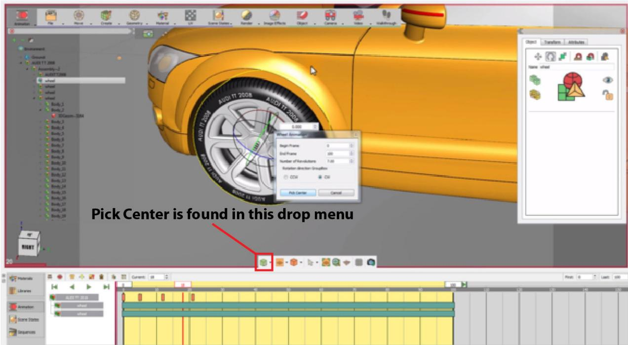
Click Pick Center, and select the circle of the tire. The normal of the circle's center will be highlighted, click the approve icon to end the process. As can be seen in the image, an animation line for the Tier has been added to the timeline.
